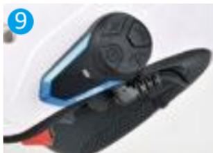
9 Adjust microphone, the installation finished.
