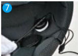
7 Remove lining, 3M glue fixes microphone
